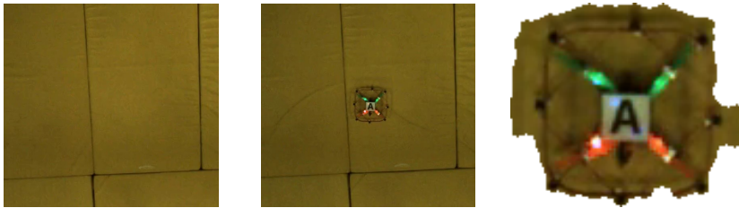
Figure 3.5: For the automatic crop an image of the background without robot (left) is recorded. It is used in a background subtraction algorithm to extract the robot crops (right) from the image sequence with robot (middle). Note that the automatic crop still contains some background due to the shadow of the robot on the ground.
