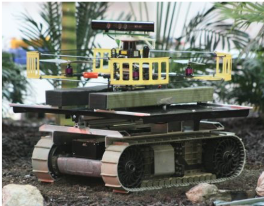
Figure 2.2: The Pelican MAV being transported by the iRobot PackBot, described by [Mulgaonkar and Kumar, 2014].
