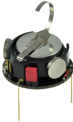
Figure 2.2: Image of the Kilobot as described in [39]
